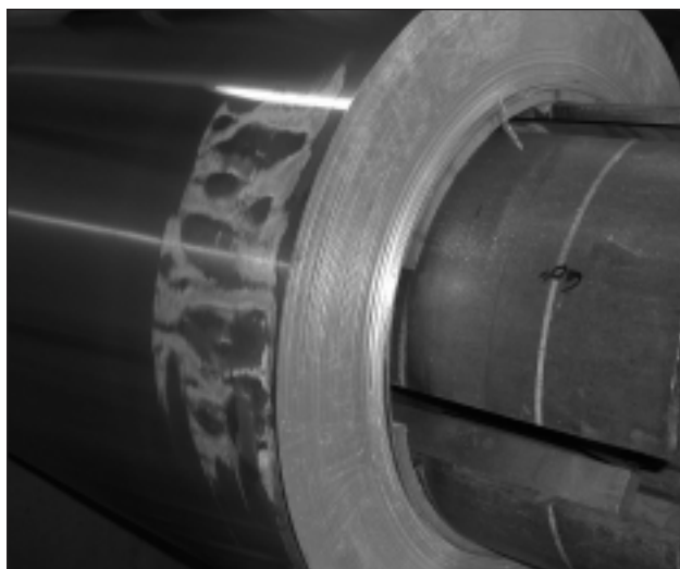
Figure 1 – Water Stain on Coil
