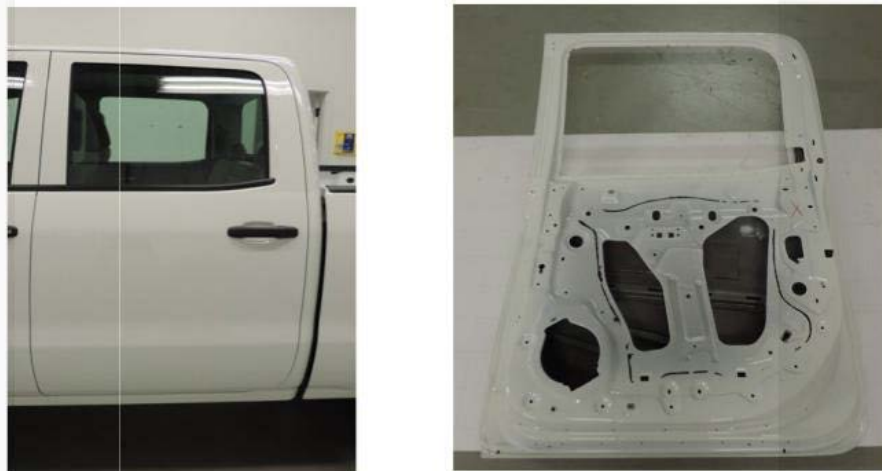
Figure 11. Baseline rear door frame (3)
