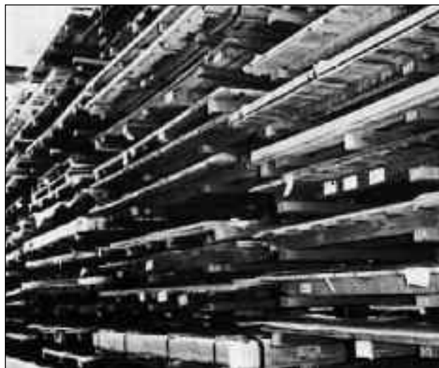
Figure 2 - Typical type of cantilever rack
