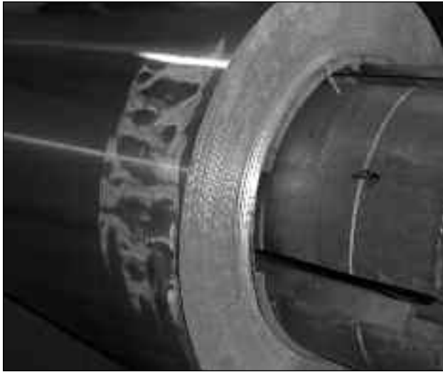
Figure 1A - Water Stain on Coil
