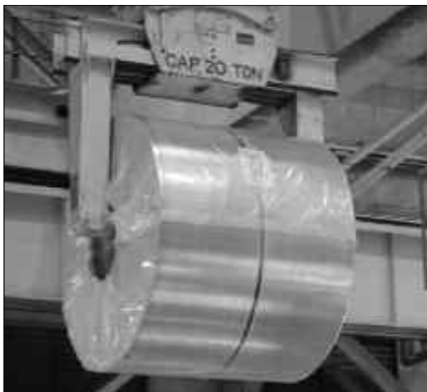
Figure 14 - Crane w/Horizontal Coil Grabs
