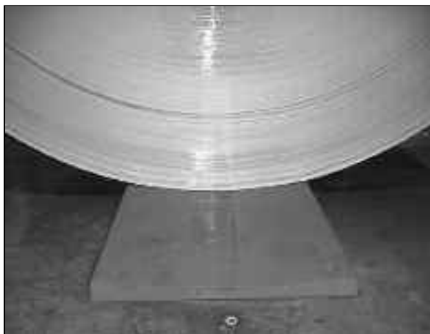
Figure 7 - (A) Storage of Coil on Protective Padding (B) Example of Wedge-shaped Protective Padding
