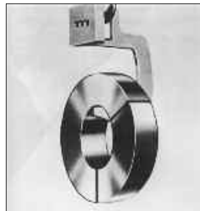
Figure 12 - Overhead Crane w/ Coil on a "C" Hook
