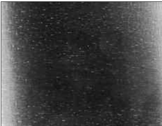
Figure 5 - Example of a Tension Scratch
