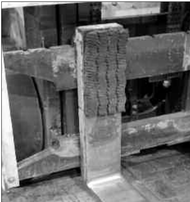
Figure 8 - Padding on Forklift to Protect Coils
