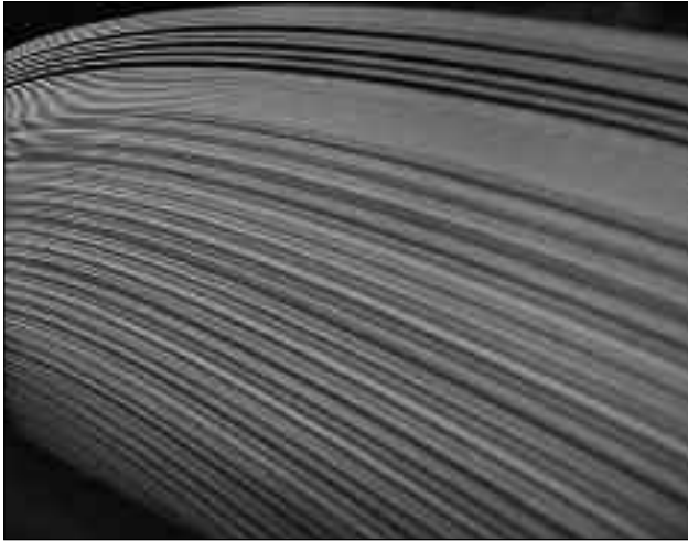
Figure 4 - Loose Wraps on a Coil
